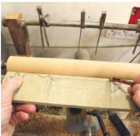
▲ Pic.16 Once you're happy with the bases, mount the stem between centres, make it round using your spindle roughing gouge and mark out the detailing on it using your template
